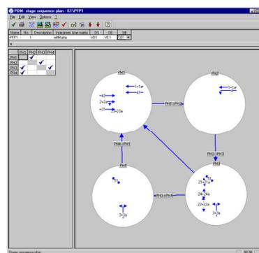
Figure 3: Stage sequencing of typical European controller [2]
