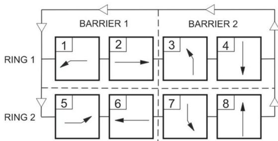
Figure 1: Dual ring eight-phase control defined by NEMA nomenclature
