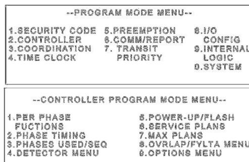
Figure 2: Example of typical 2070 controller menu programming options [1]
