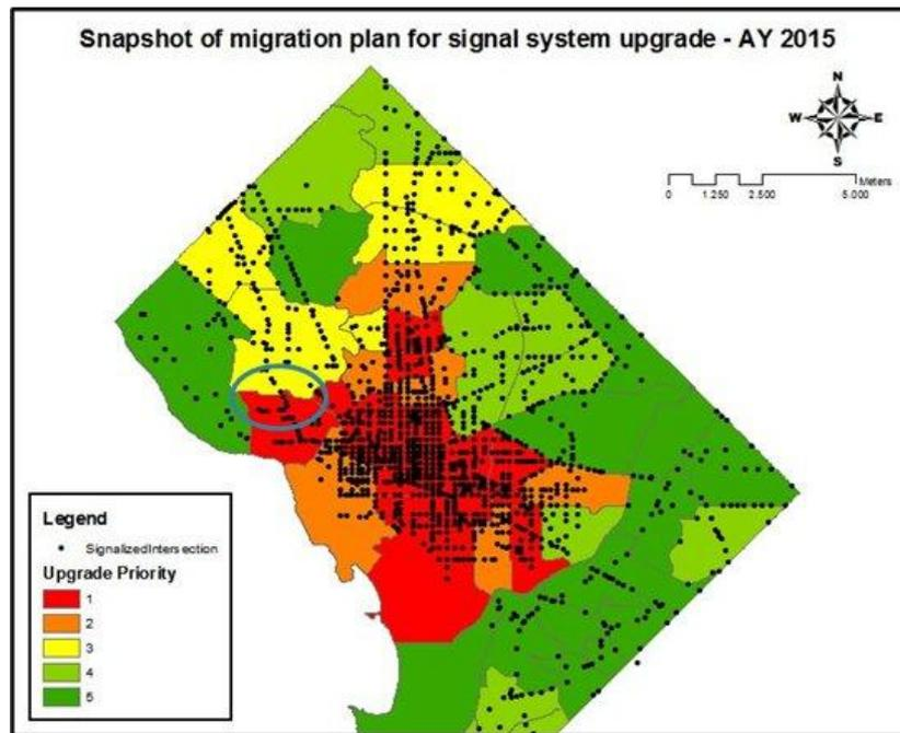
**Fig. 4** Hypothetical migration plan for traffic signal control system in the area
