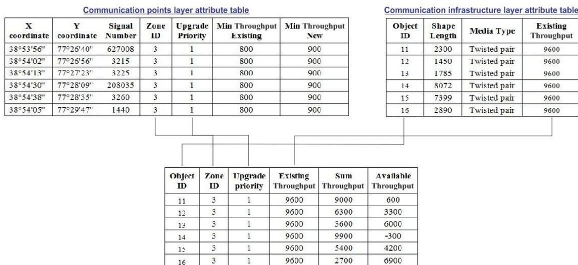
**Fig. 5** Content of final overlap layer originating from the overlap analysis related to communication points and communication infrastructure layer
